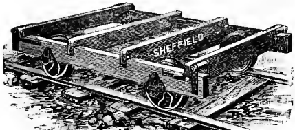
Fig. 5603. TRACK-LAYING CAR. Size, 7 ft. 8 ins. \times 6 ft. 3 ins. Capacity, 20,000 lbs. Weight, 1,300 lbs.
